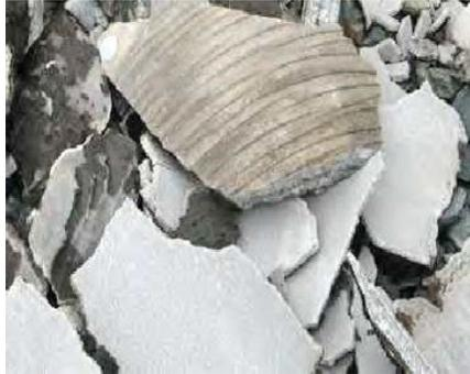
*Figure 2. Struvite Buildup Removed From Pipe*
